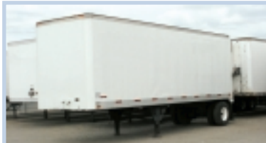
(6) 1991 Wabash 28'x102' Dry Vans w/Roll-Up Doors , Wood Floors, Pintle Hitch, Low Profile 24.5 Tires On Steel Wheels, Some Alum. Sides & Some FRPs, Translucent Roof..... $2,750 Ea.
