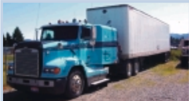
1994 Great Dane 45' Dry Van , Walco 4,000# Rail Lift, Roll-Up Rear Door, Spring Susp., Wood Floor, 2-Rows E-Track, Alum. Scuffboard, Translucent Roof, 11R22.5 On Alum. Wheels..... $6,500
