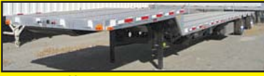
New 2006 TRANSCRAFT 51'6" x102" D-Eagle Drop Deck, w/sliding rear axle, 255/70-22.5 radials, alum. wheels, (2) boxes, sliding winches both sides, LED lights, alum. deck, 40" 6" lower deck .....$37,500 Incl. F.E.T.
